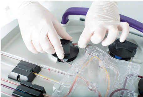
Figure 5-29a: Removing the Pump Tubing Segment
