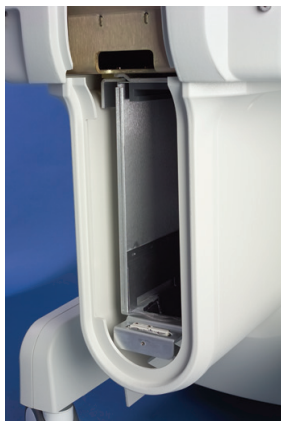
Figure 7-3: Changing the THERAKOS™ CELLEX™ Light Assembly
