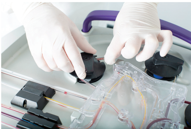
Figure 5-63a: Removing the Pump Tubing Segments
