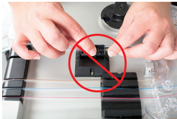
Figure 4-17b: Incorrect Handling of the Hematocrit Cuvette
