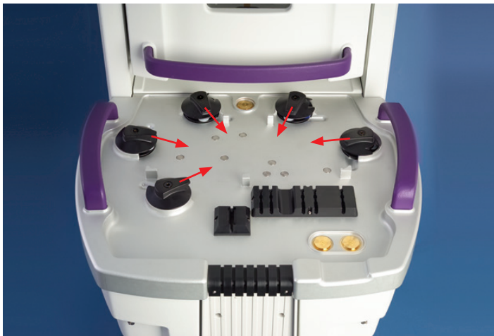
Figure 4-2d: Starting Position of Pump Handles
