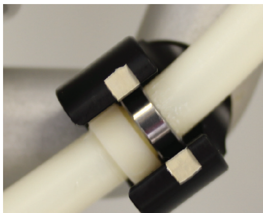
Figure 4-11b: Lower Drive Tube Bearing Installed in the Lower Bearing Retainer
