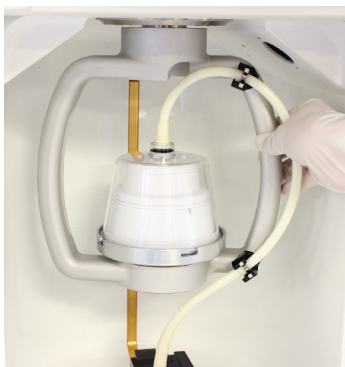
Figure 4-12c: Verifying Proper Bowl Installation
