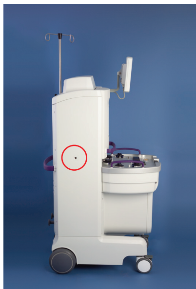
Figure 3-25: Centrifuge Chamber Door: Manual Release Access
