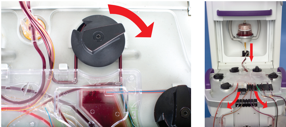
Figure 5-55: Manually Draining the Centrifuge Bowl
