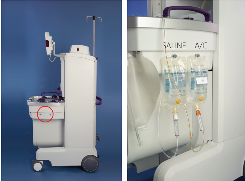
Figure 3-19: Correct Placement of Saline and Anticoagulant (A/C) Bags
