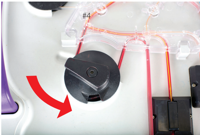
Figure 5-54: Manually Draining the Photoactivation Module
