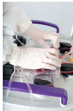
Figure 5-63b: Removing the Pump Tubing Organizer
