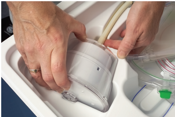
Figure 4-6a: Loosening the Centrifuge Bowl
