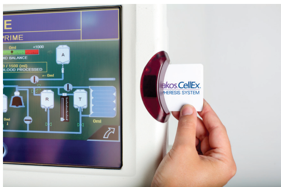
Figure 4-14b: Correct Smart Card Insertion
