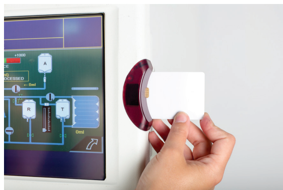
Figure 4-14c: Incorrect Smart Card Insertion
