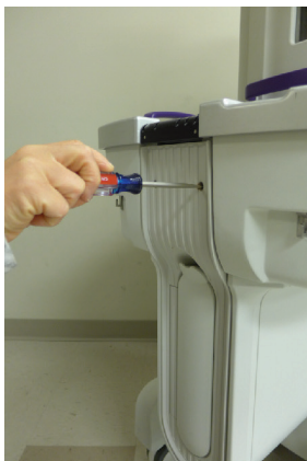
Figure 7-3: Changing the THERAKOS™ CELLEX™ Light Assembly
