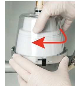
Figure 4-10g: Installing Bowl—Rotate Bowl Clockwise to Lock Clip and Counterclockwise to Confirm Centrifuge Bowl is Secure
