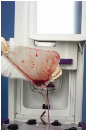
Figure 5-56: Manually Draining the Return Bag
