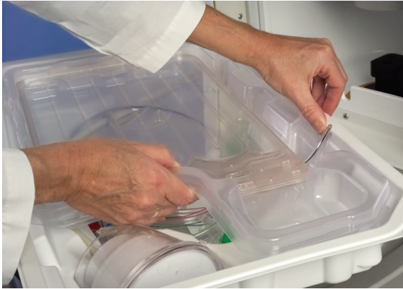
Figure 4-4a: Removing the Photoactivation Module
