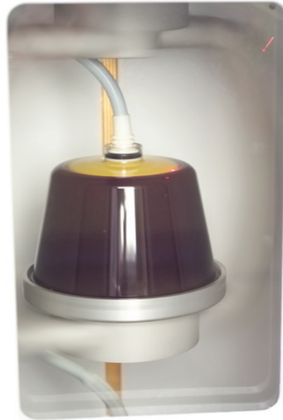
Figure 3-21b: Plasma/Red Blood Cell Interface (Actual)
