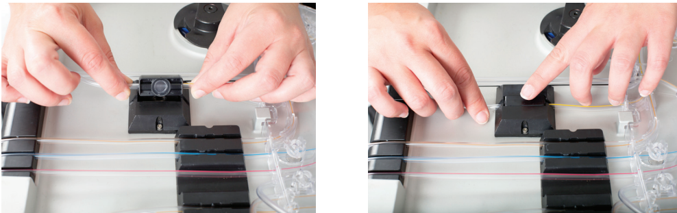
Figure 3-37: Correct: Hematocrit Cuvette Handling and Placement
