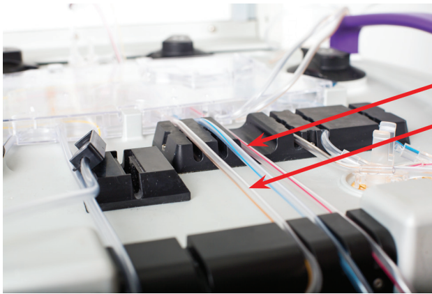
Figure 4-16b: Lines Placed incorrectly
