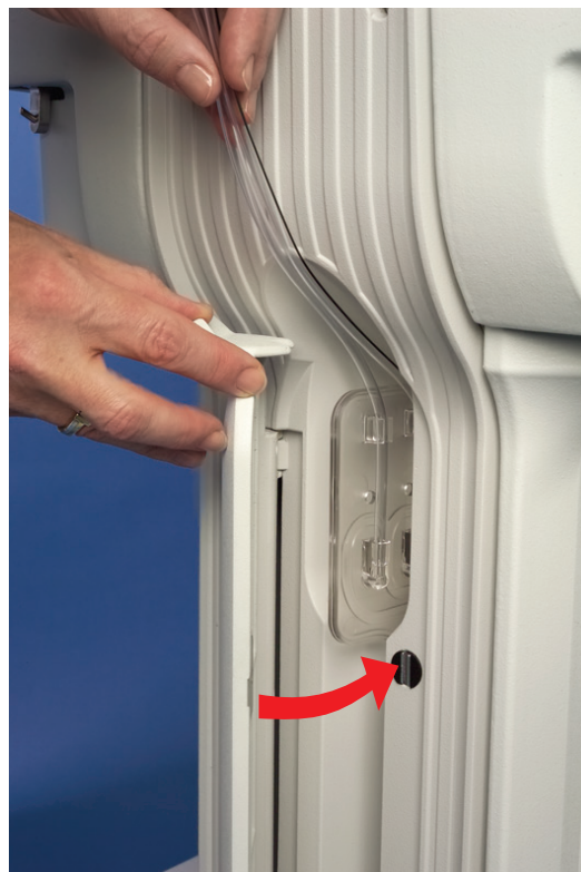
Figure 4-5b: Closing the Photoactivation Chamber Door
