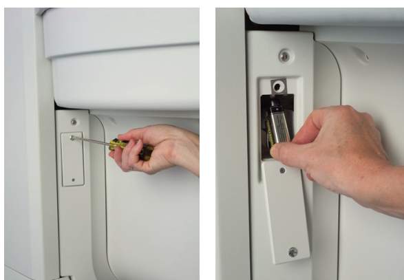
Figure 7-1b: Changing the 9 V DC Battery
